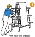
With travel lock engaged push from the seals as shown
