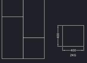
Tile construction is from 6/9mm medium density fibreboard (MDF) adhered (using water based adhesive) to 18mm sound absorbing foam.
