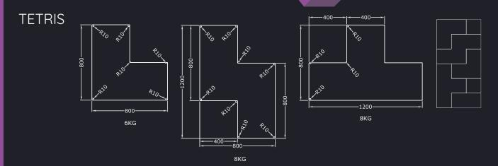
Tile construction is from 6/9mm medium density fibreboard (MDF) adhered (using water based adhesive) to 18mm sound absorbing foam.
