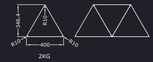
Tile construction is from 6/9mm medium density fibreboard (MDF) adhered (using water based adhesive) to 18mm sound absorbing foam.
